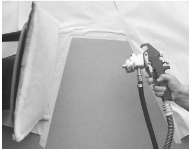
Spraying Toward Filter Hoods
