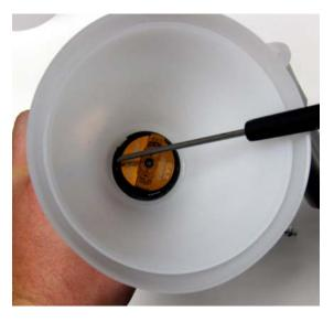
B. Insert the metal probe under the snap ring and gently lift the ring from the groove by moving the probe around the Air Cap Retaining Ring. Once the snap ring is free remove the inner and outer cones, taking care not to lose the snap ring.
